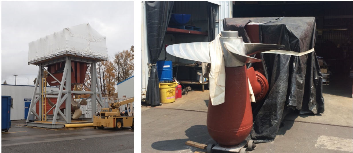
FIGURE B-4: THRUSTER OUTDOOR STORAGE AND MOVEMENT ON ITS SIDE
